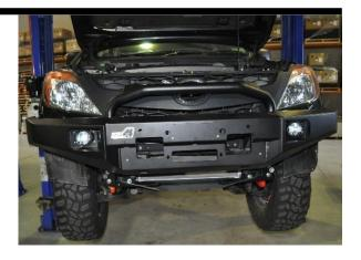
When happy with the position of the bar locate the holes in the mounting brackets that are in the middle of all the mounting bolts. Mark this hole with a white marking pen.
