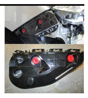
Mask off headlight and guard edge that could be seen between bar edge and body and paint black.
