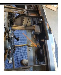
If fitting a winch to the bar, bolt it from the inside prior to bar installation on the car.
