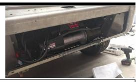
Winch mounts feet down and is installed through the front of the bar. Control boxes mount on top of winch using brackets supplied in the winch fitting kit.
