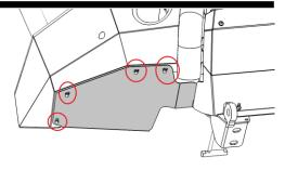
Fit centre bash plate using M8 done head bolts, flat washers and flange nuts.
