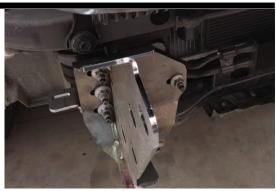
Just rearward of body mount is rectangular hole in the chassis. Slide machined bar in, with the tapped hole closest to the outside and flats facing forward. Careful to not drop inside the chassis! Slide the M10x220mm through the centre hole on the mount and engage in the machined bar.
