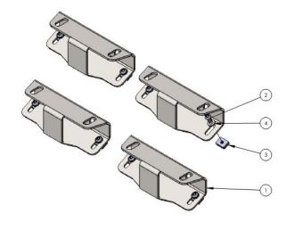
If fitting to a Ranger or BT-50 with out a roller shutter 2 reinforcing brackets are required:
