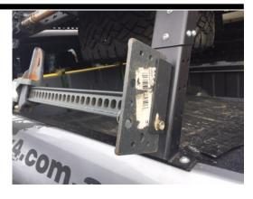
Fit Head section to other end with supplied hardware.
