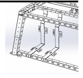
Fit box on the brackets and secure with two ratchet straps (not included.) One underneath, and one around the back, and make sure you feed strap through slots.
