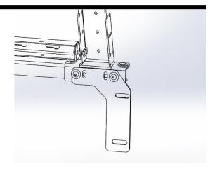
Mark each hole with a centre punch. Remove the rack and drill through each hole with a 8.5mm or 9mm drill bit.
