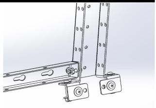
Join the Rack top section to the Rack Extension using M8 hardware
