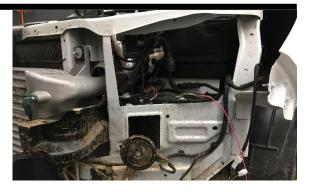
Use bumper cut template on bumper then continue the line horizontally. Refit bumper to vehicle.
