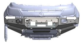
Attach outer wing guards using M6 bolts on washers to the wing, and M8 button head cap screws and M8 flat washers on the lower mount point.
