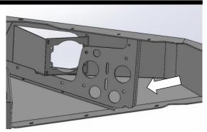
Centralize bar on vehicle first to wing then fender so clearance is as even as possible on both sides.
