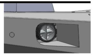
Remove remote plug from control box and install in bracket shown.
