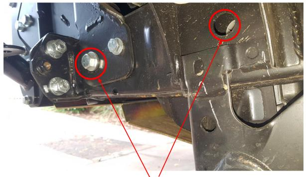
These holes in the frame are where the recovery points bolt through.
