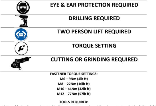
Basic tool kit, soldering iron or electrical in-line connectors, male and female spade terminals, drill and drill bits up to 12mm.
