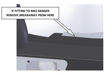
Note: Even though these bars do not require a bumper cut it will be necessary to cut the grille on the Ranger PX2 version. Mark grille as noted bellow. The grille can be taken apart in sections via removal of screws behind grille. This is recommended to make cutting easier. De-burr all sharp edges when done.
