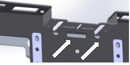
Fit lower stainless panel to bar using 4 x M5 countersunk screws and M5 flange nuts. If fitting radar to PX2 Ranger punch out grille section and drill the three holes to 8.5mm.
