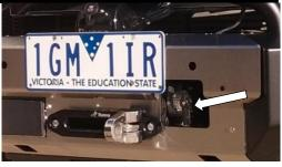
Check there is enough gap between winch rope and loom cover if tech pack model.
