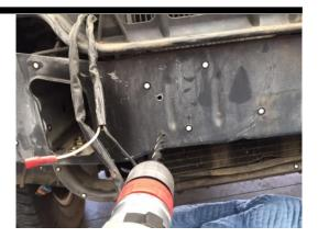
Fit impact absorbers back on to the Jeep. After the M10 bolts from the underside are loosely fit, you can feed nut plate up through access holes and feed M10 bolts spring washers and flat washer through these.
