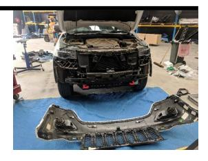
If vehicle is fitted with adaptive cruise control, remove ACC Radar unit and set aside for refitment to new bar.
