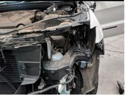
Use a test light to determine correct wires for the parker and indicator circuits.
