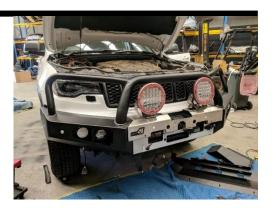
If fitting a winch do so at this point. Follow instructions provided by winch manufacturer. The design of the winch cradle spaces the winch approximately 30mm behind the front face of the bar. Depending on the length of fasteners supplied by the winch manufacturer, longer fasteners may be required. ALWAYS use high tensile (GR8.8 or above) fasteners when mounting winch.
