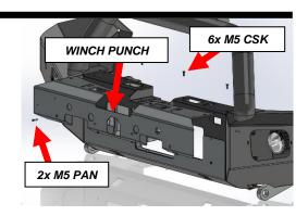
Fit front fascia to bar using M5 countersunk screws and flange nuts provided. As the fascia is offered up to the bar, insert the parking sensors into their respective housings mounted to the fascia.
