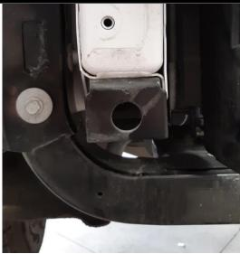
Remove small protruding bracket using grinder. Paint bare surfaces when complete to prevent corrosion.
