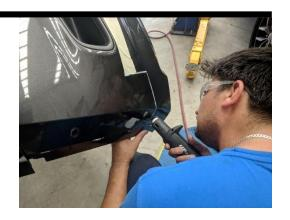
Once complete re-fit top section of bumper to vehicle. Fit pinch weld to end sections of bumper where cut will be visible.
