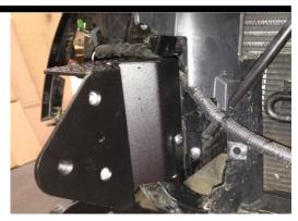
Fit radiator support rod brackets to impact absorber using M6 fasteners, flat washers and flange nuts provided.
