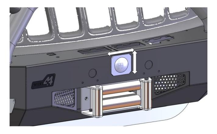
Remove clips and screws holding wheel arch guards, flares and center stone guard to vehicle bumper. Disconnect fog lights, parking sensors and ACC/radar if fitted. Retain all clips and screws.
