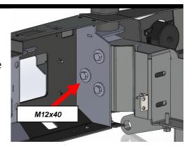
Align the bar so the top surfaces or tops of wing edges are parallel to the rake angle of the vehicle. Adjust the bar to the final position and tighten all mounting bolts.
