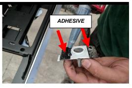
Fix the sensor housing to the inside of the bull bar and top fascia panel in the same position they were removed. No.2 and No.5 are rotated 180 degrees. All others are rotated as removed. Leave adhesive to cure for at least 1 hour whilst continuing with other steps.
