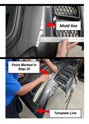
Re check all measurements. Carefully cut along marked line in bumper with air reciprocating saw or angle grinder. De-burr edges if necessary.
