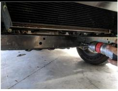
Refit under panel and secure to bull bar with M8x25 Button head bolts and flat washers.
