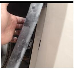
With the bonnet open remove all clips holding the top of the grille on.
