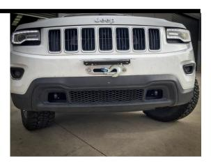
If fitting an ACC radar camera, you must remove it from the factory bracket and screw it into the Uneek bracket with M5 hardware then mount it to the pre runner.
