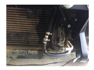
If fitting the optional hidden winch mount, place the mount between the RH and LH impact absorbers and loosely fit all bolts including top gusset as shown.
