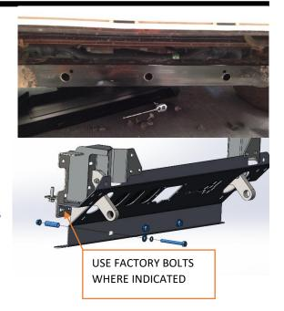
**Note:** For reference these holes are 25mm up from the bottom lip, the middle one is in the center and the outside ones are 200mm each side.
