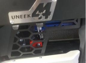
Fit Jack points using M8 button head bolts and black flat washers.
