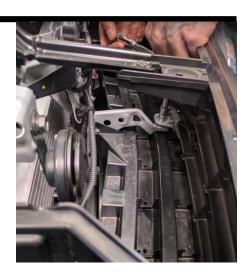
Remove clips holding bumper on. Clips are located in wheel arch and under the vehicle.
