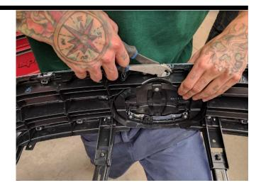
Clip on grille retainer bracket and refit to car.
