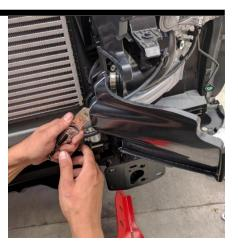
Mask off headlight and panel and paint edges of panel and headlight which could be seen between bar and body black.
