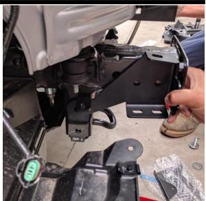
Fit red chassis mounts to each chassis end.
