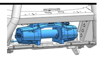
Winch mounts feet down and is installed through the front of the bar.
