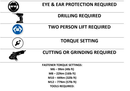
BASIC TOOL KIT WITH SOCKETS, SPANNERS AND HEX KEYS, Power drill with 5mm and 9mm drill bit, rubber mallet, centre punch, hammer.
