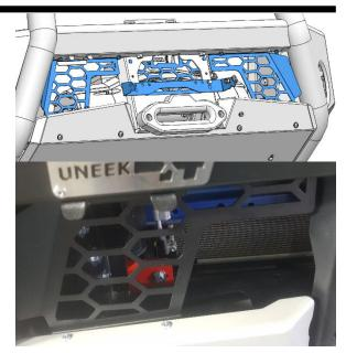
• Fit Jack points using M8 button head bolts, black flat washers.
