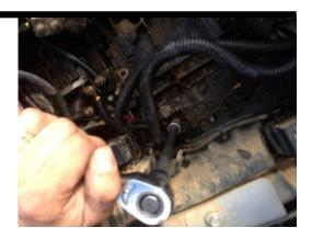
Remove the bolt on the bonnet seat edge as shown in the right.
