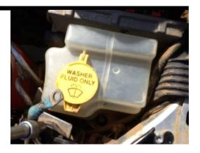
Remove the bolt at the bottom of the washer bottle. This is accessed from the top.
