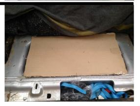
From the edge of the rubber measure 168mm in. Mark a line and this will be the edge of the cardboard cut out. Trace a line all the way around the cardboard cut out and remove the cardboard.
