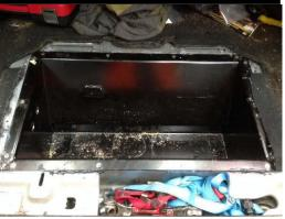
If fitting a battery use clamps and bolts supplied to clamp down batter to tub. Feed battery cables through supplied cable glands.
