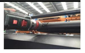
Fit M10 x 70 button head cap screw with nyloc nut and washer and torque up.
