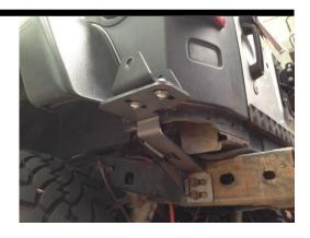
The picture to the right shows the ideal spot for the chassis brackets, which is 40mm from the edge of the body and 40mm from the flare at that point from the body.
