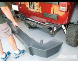
Remove the two steel side brackets from your plastic bumper.
