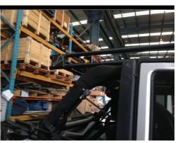
Attach the front of the roof rack to the front hoop with 2 x M12 hand knobs. Make sure you use a spring washer and flat washer as well.
