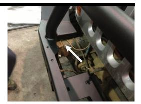
If no winch is installed, an optional winch delete plate can be installed
