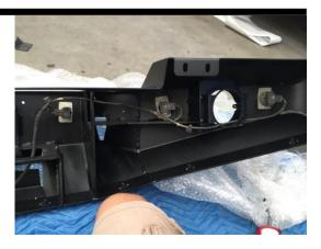
Apply a small bead of adhesive silicon to the front plastic mounting face of the sensor housing.
