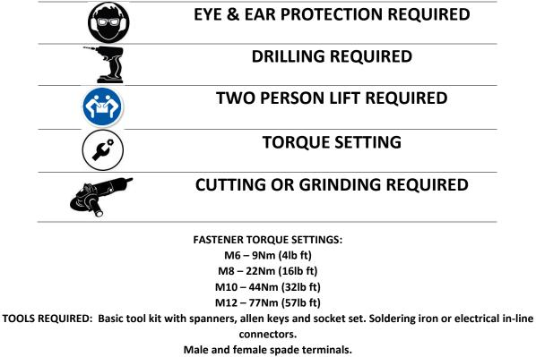
Power Drill, 11mm and 13mm drill bits, centre punch and hammer. Black adhesive silicone.
