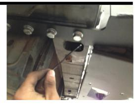
Torque up M10 x 30 bolts on the front face of the frame.
