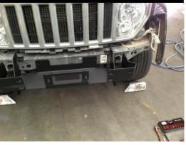
This picture shows the bolts on one side holding the winch cradle in place.
