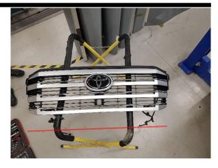
behind the rear edge of the bar so it is recommended to cut it a little lower than the bars rear edge.
