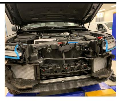
• Remove intercooler air damns (retain) and lower crash bar plastic cover (not required later).
