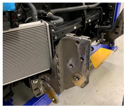
installed back off the bolts slightly to allow the mount bracket to move side to side.
