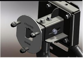
If fitting single jerry can holder in high version insert hooks into the back plate and bolt holder to the swing arm using M10 hardware.
