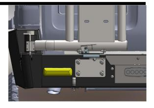
Fit striker pin finger tight and leave M12 button head cap screws loose at this point. Fit latch to swing arm with M6 hardware. Swing arm into closed position to line up the latch. Raise/lower striker pin plate and move pin left or right until there is a clean opening and closing feeling. Torque all bolts once that is achieved.
