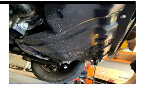
Remove the radar sensor and carefully store in a safe place to be reinstalled on the bulbar later.
