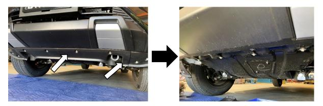
Remove all plastic trims underneath the bumper and detach the bumper from the vehicle.
