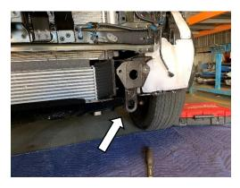
Remove the front bumper brace and the factory tow point on the passenger side.
