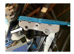
Remove and discard the brackets which supports the factory bumper on both sides.
