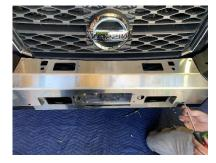
Complete all wiring before fitting stone guards. Fit middle stone guard to bar ONLY using M8 button head cap screws and flat washers. Fit original bash plate to vehicle using REAR holes only. Secure middle panel through original bash plate and into slotted hole on chassis bracket using M8 cap screws, flat washers and M8 flange nuts.
