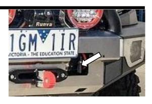
With the help of another person lift bar onto vehicle and secure using M12 x 30 bolts, spring washers and large flat washers. Make sure area shown by arrow has a minimum 15mm gap.
