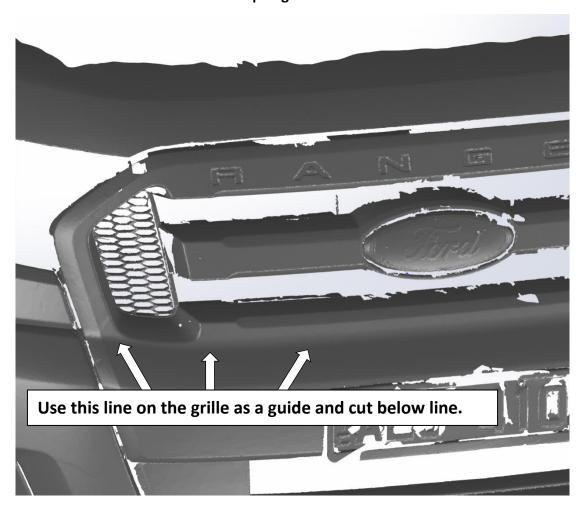
Remove plastic panels under bumper, bumper, fog lights if fitted, grille and steel bumper support. Remove plastic bumper mounts from guard sections. Retain bolts from bumper support. Remove front bash plate.
