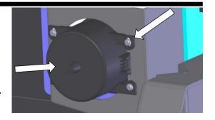
Install optional winch light and route cable to either side of bar. Run cable through access (arrow) hole.
