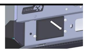
Fit under headlight brackets to wing loosely with M6 x 20 bolts, flat washers and M6 flange nuts. Ranger Mark 2 shown. Note from above parts list drawings there are two types. PX1 and PX2. PX2 is shown.
