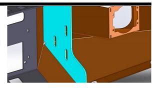
At this stage cut the PX2 grille using the larger image at start as a guide. De burr when complete and fit back to vehicle.
