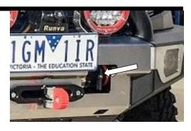
Note: Check there is enough gap between winch rope and loom cover if tech pack
