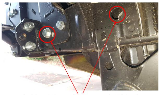
These holes in the frame are where the recovery points bolt through.
