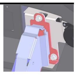
After securing winch cables etc mount centre stone guard to bar using M8 cap screws and M8 flat washers. Secure to chassis with M8 x 40 bolts and M8 flat washers. NOTE: The spacer tubes are mounted between the supplied guard and the Toyota guard. When all bolts are in tighten.
