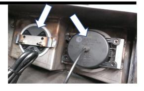
Install optional winch light (Narva 90862) and route cable to either side of bar. Run cable through access (arrow) hole and cable tie to holes provided.
