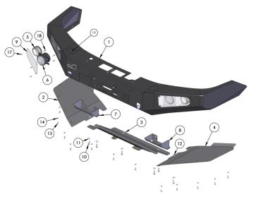
Remove plastic panels under bumper, bumper, fog lights if fitted, grille and steel bumper support. Rove two front bolts from lower steel bash plate and retain. Loosen other bash plate bolts only.
