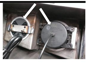
Install optional winch light and route cable to either side of bar. Run cable through access (arrow) hole and cable tie to holes provided.
