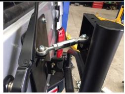
Note: over time as the stop wears you will need to re-tension the tie rod.
